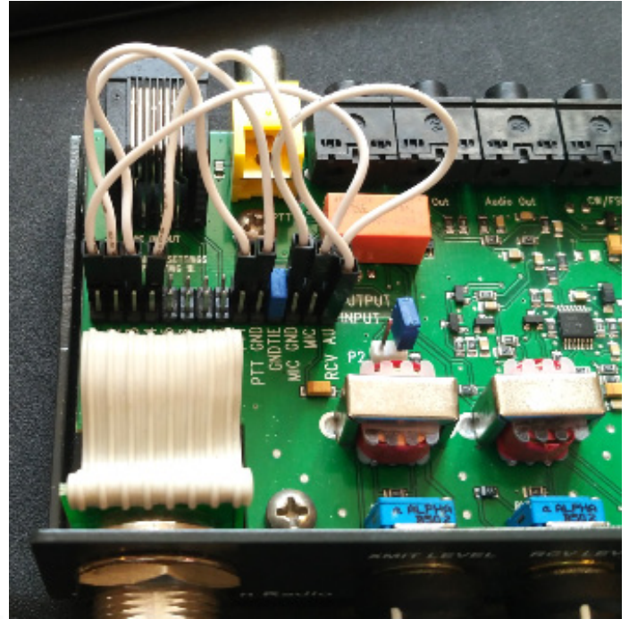
The completed jumper wiring for 9k6 audio.
