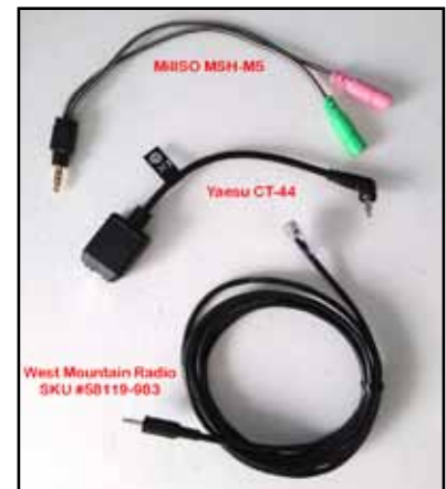
Figure 4: The cables and adapters required to interface to the Yaesu FT-250R
