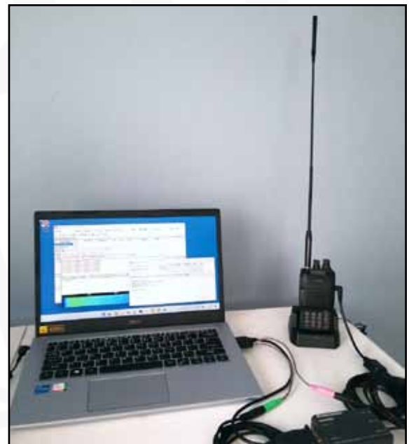
Figure 3: The completed WL2K station
