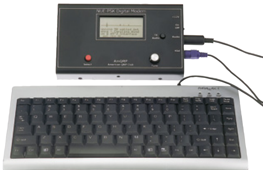
The NUE-PSK modem sends and receives PSK-31, with more modes to come, without requiring a computer. Any PS/2 keyboard can be used. The NUE-PSK is shown here with the lightweight, portable Parallax Mini-Keyboard, which is available from retailers for $19.95 (or directly from Parallax at www.parallax.com ).
