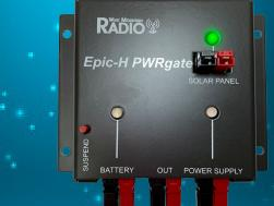
Charge the Battery -Solar Panel Input
