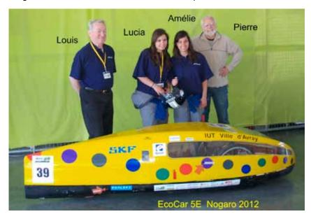
A multi-year effort, EcoCar 5E was designed in accordance with rules for the battery powered (only), all electric prototypes for the EducEco Challenge competition. It finished the 2012 competition in 5th place at Circuit Paul Armagnac in Nogaro, France. This body was originally constructed for different class, powered by an internal combustion engine.
