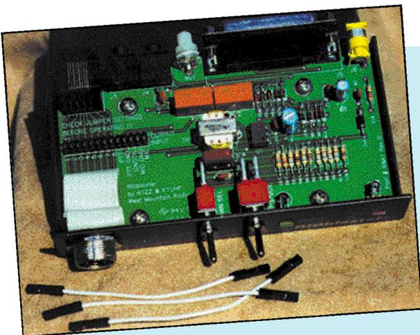
Interior view of the RIGblaster, with three of the jumpers you'll need to install on the left side. Arrangement of the jumpers varies with the type of radio you're using.
