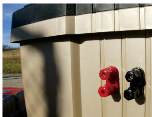
These female banana plug posts can be used to export power to external chargers, or to import power from a 12v source such as your car battery.
