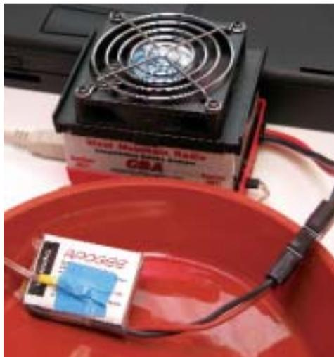
Securely tape the temperature probe to a Li-Poly battery. This holds the temp probe in place and isolates it from the cooling effects of the surrounding air. A magnetic tip in the probe holds it against the metal cell walls of nickel batteries.
