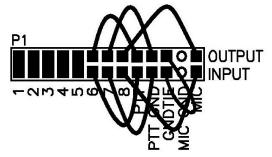
Note: If your radio's manual shows only 1 ground pin on the mic. connector you have this style. Notice the wire jumper on our GNDTIE pins.
