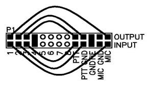
Note: There is a 2 pin jumper on the GNDTIE pin as Ten Tec uses a common mic. and PTT ground.
