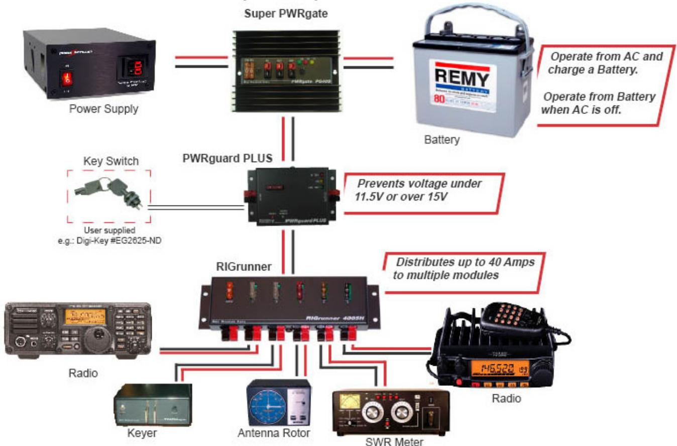
PWRguard Plus will automatically turn the power off when its input voltage exceeds 15 volts or drops below 11.5 volts. Momentary dips below 11.5 volts are tolerated to prevent false tripping. Custom trip limits now can be programmed to suit a customer's specific needs; for example to accommodate different battery chemistries, cabling voltage drops, or a rig's input power requirements.
