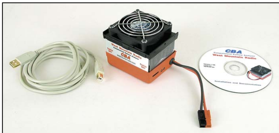
Figure 5—The Computerized Battery Analyzer consists of a heat sink and small fan sitting on top of a plastic tray.
