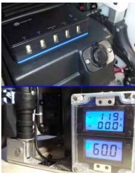
To minimize stray power electronics and cables cluttering my life, the machine includes three independent USB charging sources totaling 8 outputs, AC metering, a “cigarette lighter” 12-volt outlet, spade terminals on the battery, a utility board with barrier strips, a cable for charging the network slice of my backpack, and a charger for AA and AAA batteries.
