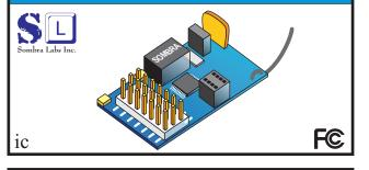
Sombra Labs proudly introduces the Shadow-3 Receiver, the world's smallest and lightest 7-channel full-range, fully-synthesized "crystal-less" receiver. This compact, lightweight, ultra-narrowband receiver for RC aircraft, cars, and boats can process up to 14 PPM channels and seamlessly cover 72MHz (air) and 75MHz (surface) bands.
