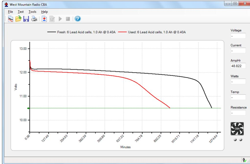
Battery degradation makes it extremely important to test your battery at regular intervals, usually every 3 months, to ensure your equipment will be protected when there is a power outage and the need for emergency communications.
