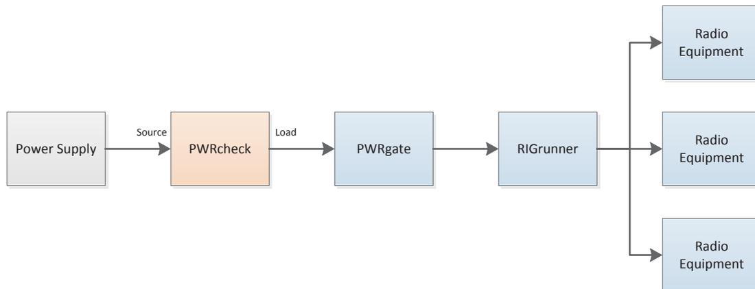
3. Turn the power supply on and set it to provide 13.8V DC. The PWRcheck will turn on, displaying the voltage produced by the power supply on the screen.
