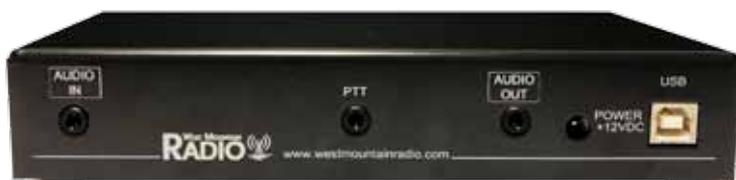
**AUDIO IN:** 1/8" stereo jack that accepts audio from a low-impedance external speaker jack or headphone output jack typically found on Amateur transceivers. Use the supplied stereo patch cable to connect to the radio if the radio has a stereo output. If using two radios, use a right/left splitter adapter or audio splitter cable to connect to two radios/audio sources.
