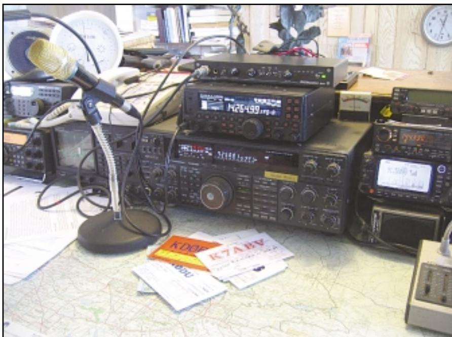
Photo A— The RIGblaster duo set up on top of WB6NOA's FT-450, one of more than a half-dozen two-radio combos he would test out through the duo from West Mountain Radio. (Photos by the author unless otherwise noted)
