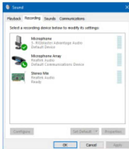
Right-clicking on the RealTek device allows it to be set as the default communication device.
