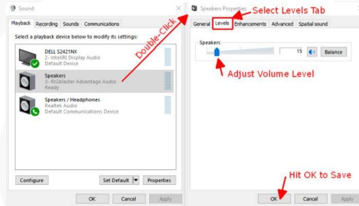
I find a value of around 10-15% is about right for modern radios with a RIGblaster Advantage but you may need to experiment a little with your particular set up.
