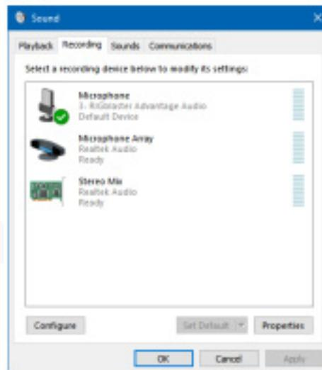
Currently you can see that the Advantage is set to be the default recording device. This is usually fine left as is but if you do use VoIP software you will want to make another device the default communications device.
