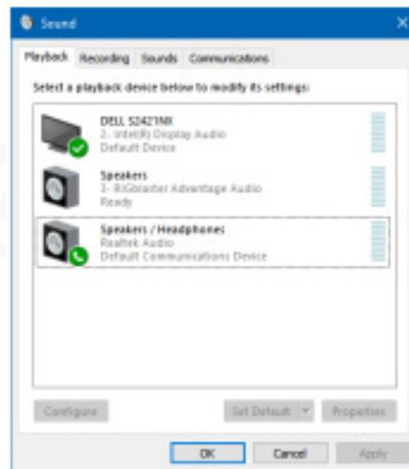
Now we can see that the Dell is the default device and the RealTek is the default communications device. There are no longer any icons on the RIGblaster device which is exactly what we wanted to achieve. This means that only the software we specifically configure to use the RIGblaster will have access to it.
