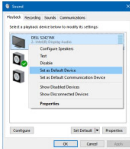
If we right-click over the Dell device we get a pop-up menu with an option to make it the default device instead of the RIGblaster.
