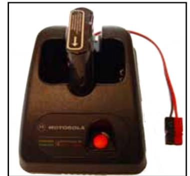
The particular charging stand chosen, the enclosure snaps together, making disassembly not requiring any tools. To prevent the charging circuitry from affecting the results of the battery test, the battery contacts were disconnected from the charging circuitry by cutting circuit board traces. Be sure to neatly cut the traces. This will make it fairly easy to add jumper wires so the charging circuitry can be reconnected in the future if desired.
