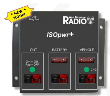
ISOpwr+ is a high powered solid state switch designed for automotive applications with or without an auxiliary battery. ISOpwr+ prevents radio equipment from draining the vehicle battery and charges the auxiliary battery while the vehicle is running. Equipment is powered from both auxiliary battery and alternator while vehicle is running.
