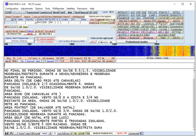
**Figure 5:** MultiPSK Decoding a Pactor Transmission
