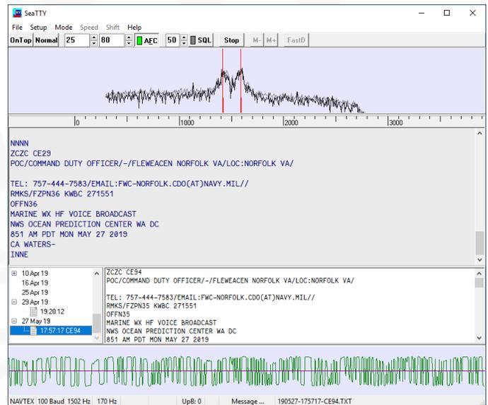
**Figure 2:** SeaTTY Decoding a SITOR-B (NAVTEX) Transmission
