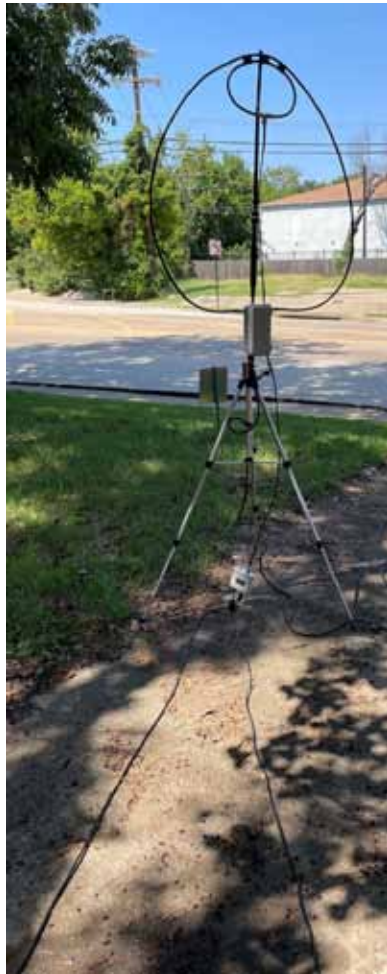
Alpha Loop showing cables separated from each other.
