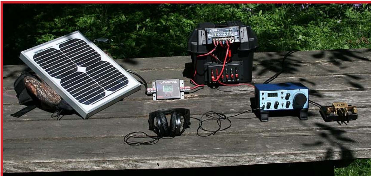
In the photo: 1) HQRP 10W Monocrystalline Solar Panel 2) Wilderness Sierra QRP Transceiver, Sony Noise-Cancelling Headphones & Kent Twin Paddle Key. 3) West Mountain Radio PWRcheck. 4) West Mountain Radio “U1 Battery Buddy DC-to-GO Box w/ RIGrunner 4005” & Morningstar SunSaver 6 Solar Charge Controller.
