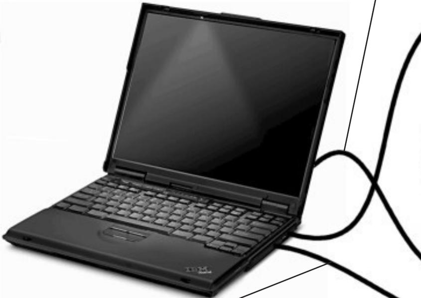
**TRANSMIT AUDIO:** Supplied 3.5 mm, 1/8" stereo phone plug audio cord from computer's headphone\* output to RIGblaster's audio in.
