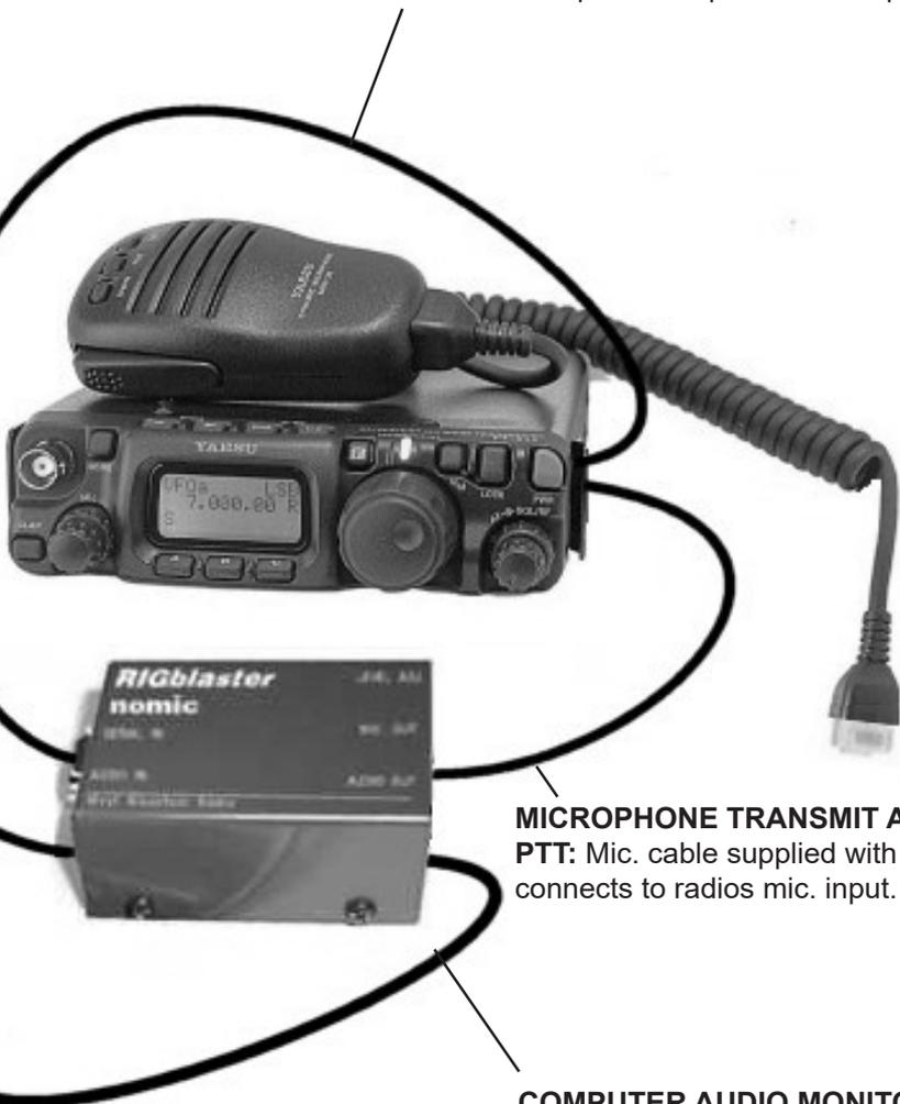
**MICROPHONE TRANSMIT AUDIO & PTT:** Mic. cable supplied with RIGblaster connects to radios mic. input.
